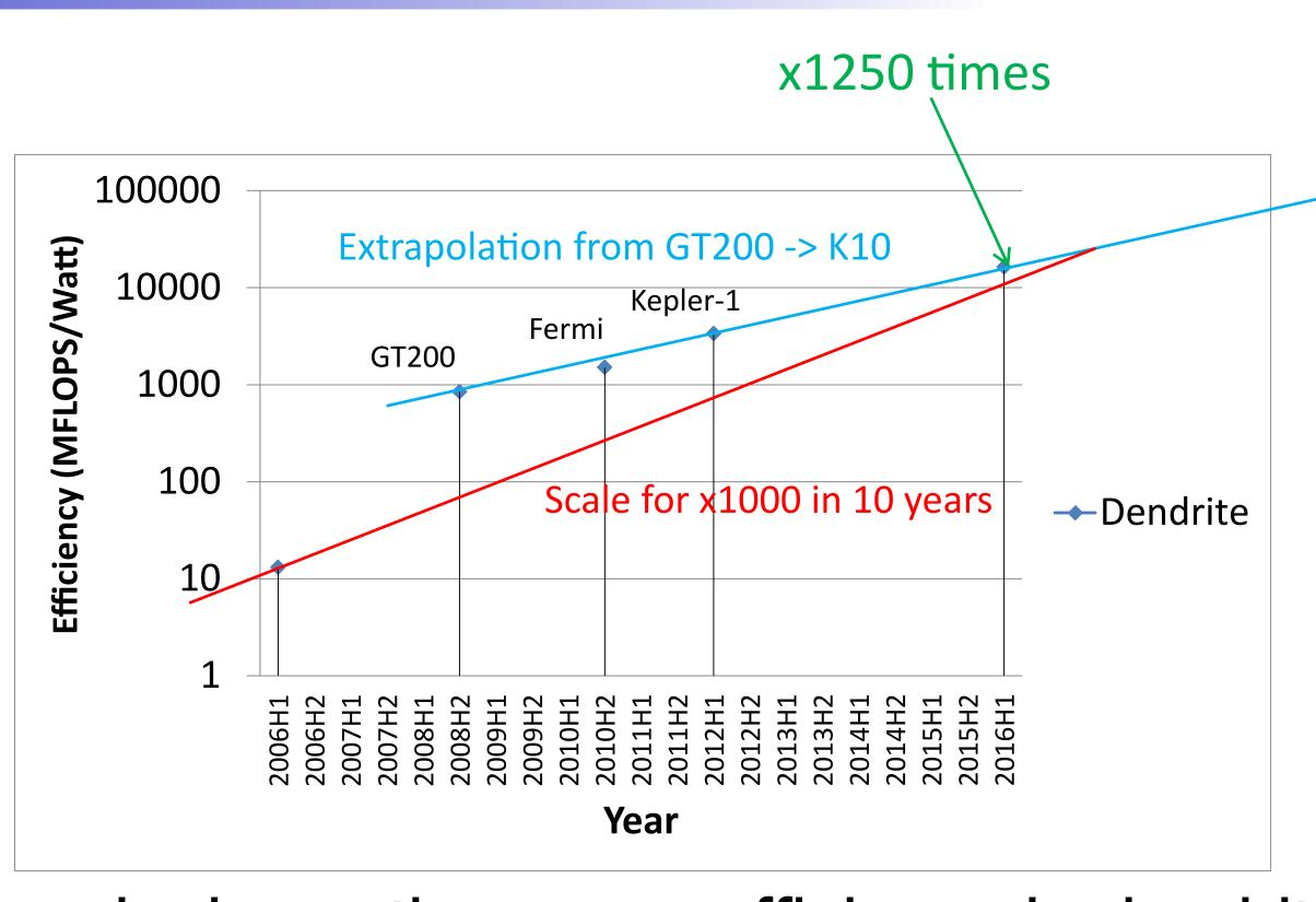
This graph shows the power efficiency in dendrite solidification simulation code (See Gordon Bell panel for detail). 2006H1 machine has only CPUs. In 2008H2, the system with GT200 GPU achieves 60x improvement. After that, GPU changes to Fermi and Kepler, which provide us higher power efficiency without any code change. Using extrapolation, we will achieve 1,250x power efficiency in 2016H1.
