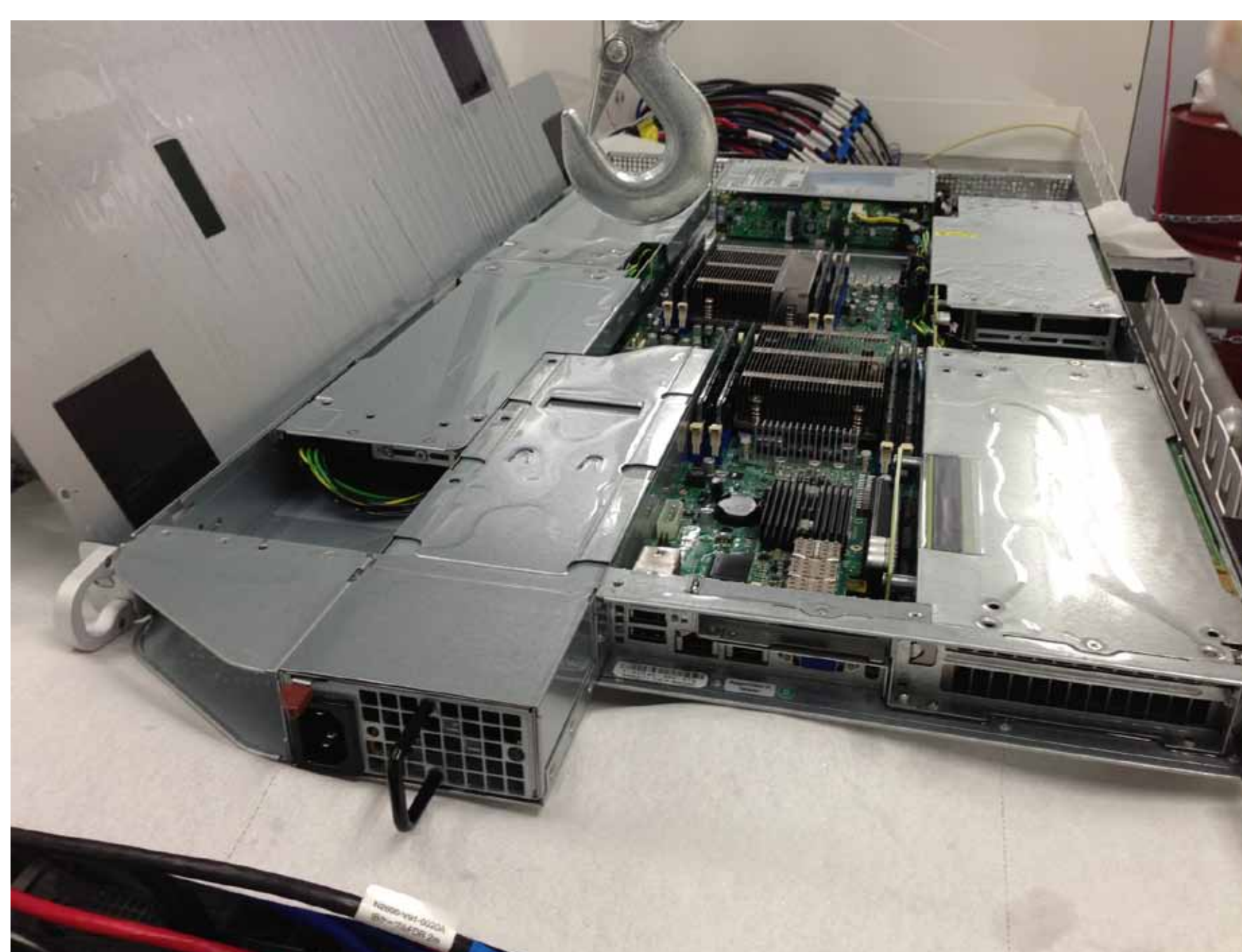
A compute node after oil-submerged
