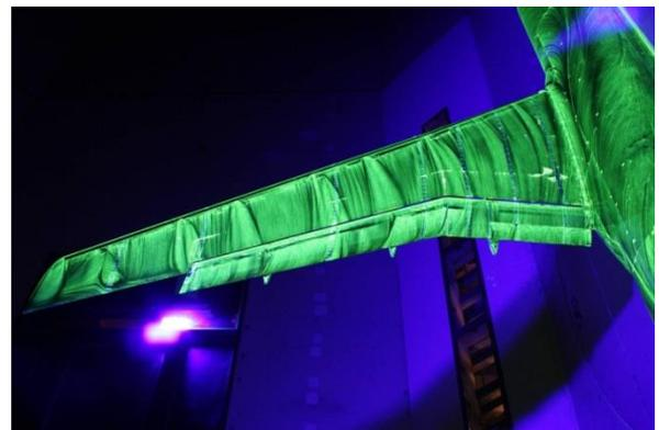
Fig.5 Surface flow pattern by Experiment
