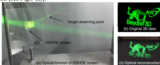
Fig.3 Optical function of DDHOE screen and the optical reconstruction of projection-type holographic 3D display
