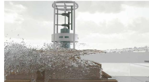
Tsunami impact pressure analysis for coast area buildings is conducted with a goal of high accurate safety estimation. Volume of Fluid based finite difference method is applied to calculate the incompressible two phase flow. AMG-BiCGSTAB is applied to solve the
