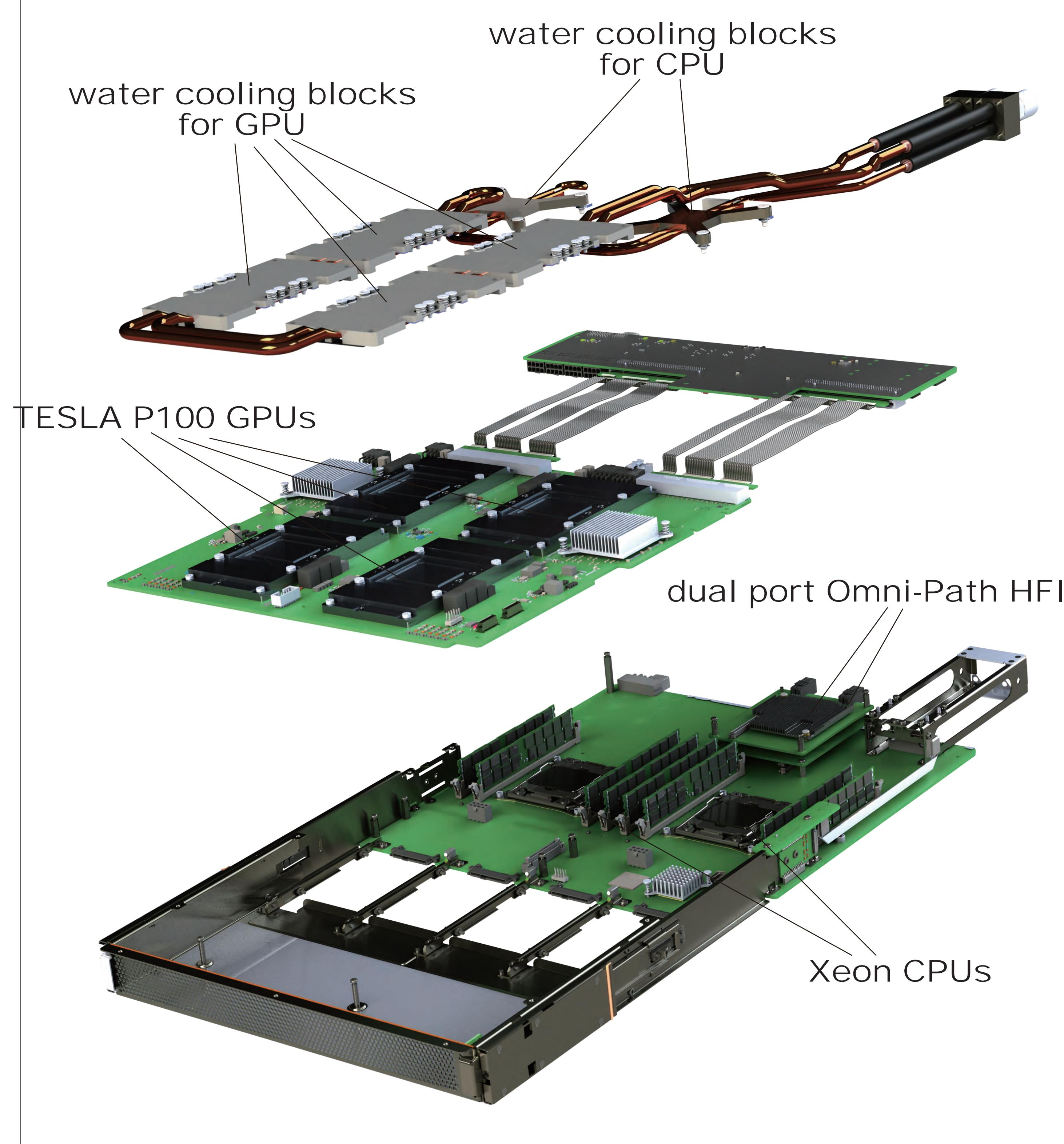
Compute node consists of four layers: CPU and Memory on 1st, OPA HFI (connected to CPU) and GPU board on 2nd, OPA HFI(via PLX) on 3rd, and Power board on 4th.
