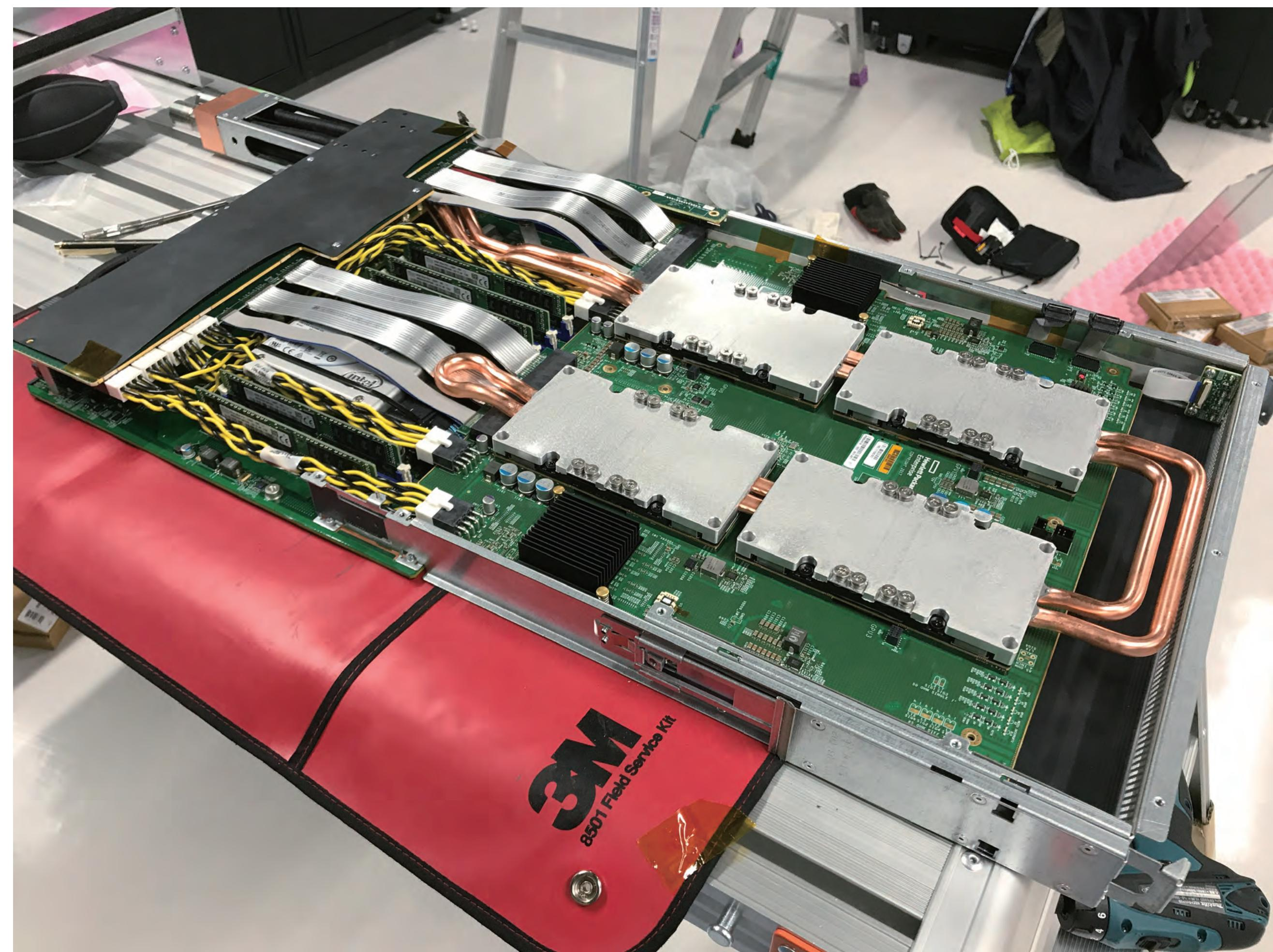
TSUBAME3.0 compute nodes are designed for HPC, BigData, and AI workloads which require all of computing power, memory bandwidth, network interconnect, and local storage. All of these components are densely installed in a compact blade using water cooling.
