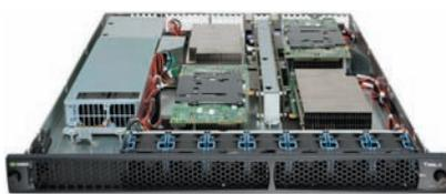
Figure 3 NVIDIA Tesla s1070 GPU retrofitted to TSUBAME1
