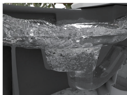
Figure 10 Real case simulation of sanitary set by TSUBAME 2.0 supercomputer.
