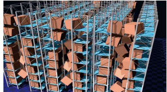
Figure 5 Simulation of falling objects from racks during an earthquake
