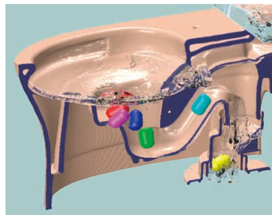
Figure 6 The simulation results of the multiphase flows containing gas, liquid and solid.
