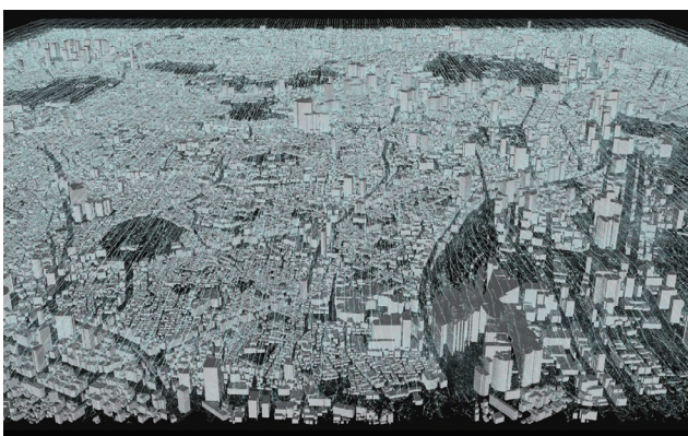
Fig. 5 Snapshot of wind flow using particles (north is up).
