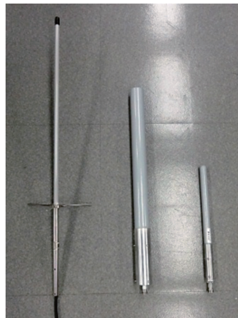
Fig. 2 Prototype transmitting antennas (from the left: 700-MHz band, 1.2-GHz band, 2.3-GHz band)
