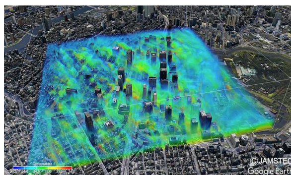
図 2 (Fig. 2) : Example of MSSG urban micro-meteorology simulation. Three-dimensional distribution of instantaneous air temperature for 13:30 JST on 11 August,
