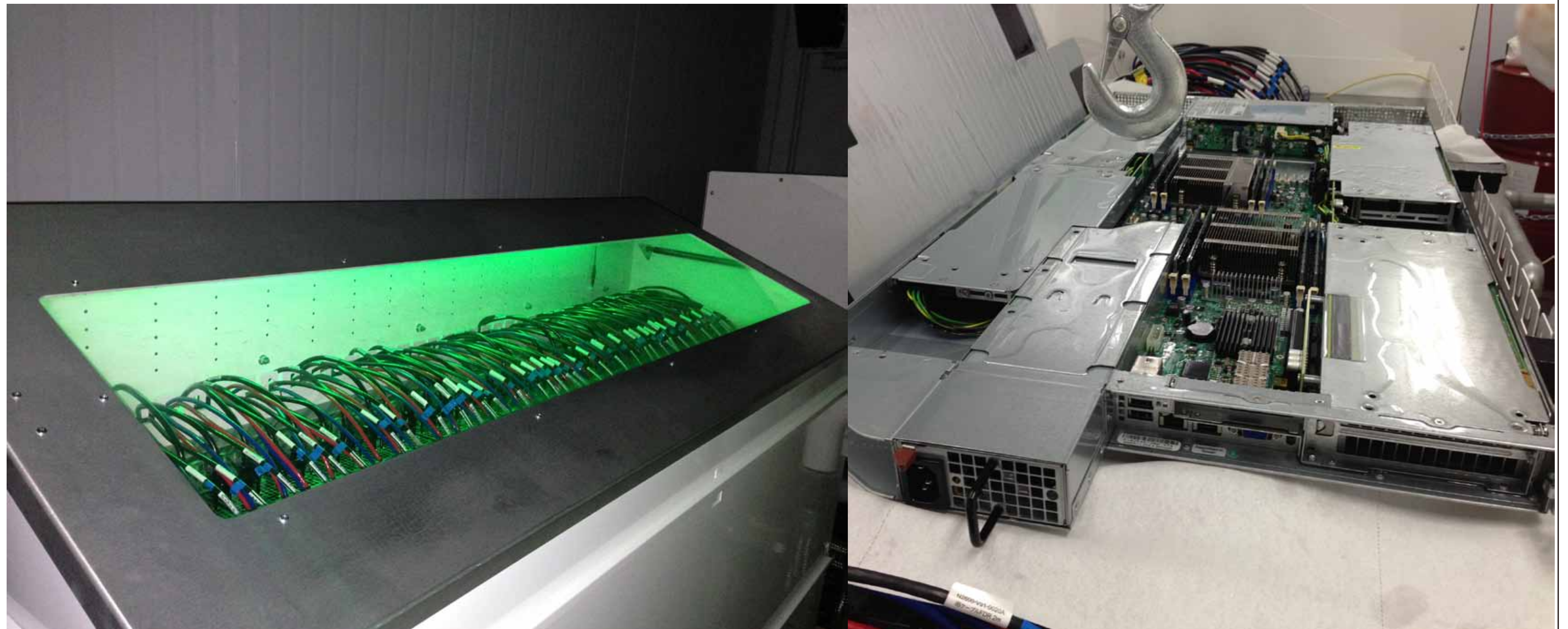
Green Revolution Cooling's CarnotJet system 42U Rack
