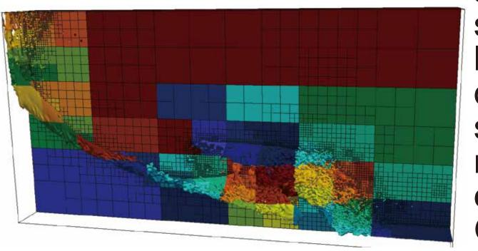
By using the adaptive mesh refinement (AMR) method, which dynamically adapts high-resolution grids to interfaces, computational cost and memory usage are educed. The spatial distribution of a computational load change in time; therefore, dynamic domain partitioning using a space-filling curve is introduced for multi-GPU computing to assign an equal number of grid points to each GPU. The figures show the
