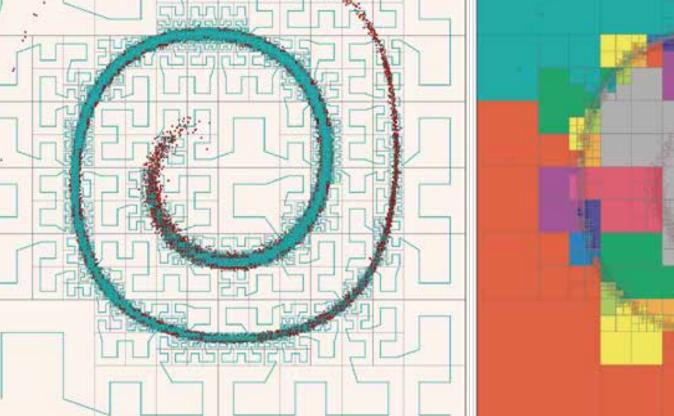
partitioning in terms of a space-filling curve(SFC) is one of promising candidates and it is recognized that a 1-dimensional mapping of 3-dimensional space by cutting the equal length. Due to low cost of SFC domain partitioning, it is suitable for frequent re-partitioning in the simulations of unsteady phenomena.
