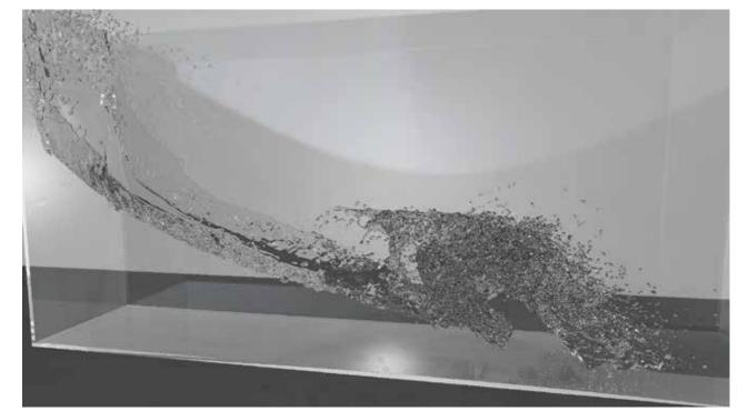
Simulations for multi-phase flows require high-resolution grids to capture phenomena at the interface.
