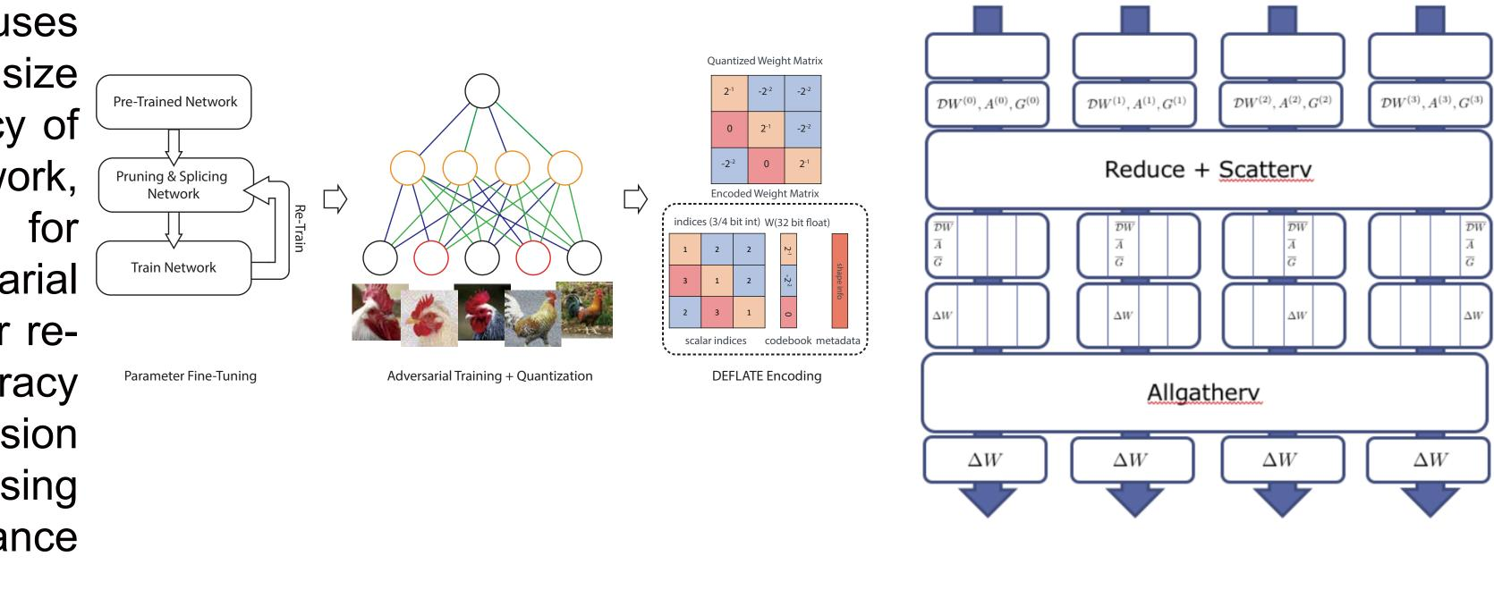
Second order optimization methods require the communication of the Hessian matrix. The present method reduces the communication significantly through Kronecker factorization and the use of reduce-scatter and allgather collectives to swtich between data parallel and model parallel execution. The optimal implementation of all reduce operations has the same communication pattern, so the present method simply inserts the computation of the Hessian.
