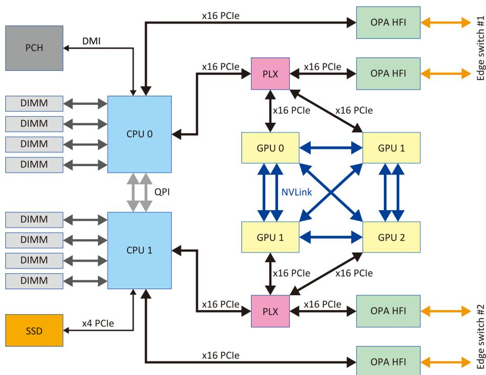
Compute node consists of four layers: CPU and Memory on 1st, OPA HFI (connected to CPU) and GPU board on 2nd, OPA HFI(via PLX) on 3rd, and Power board on 4th.
