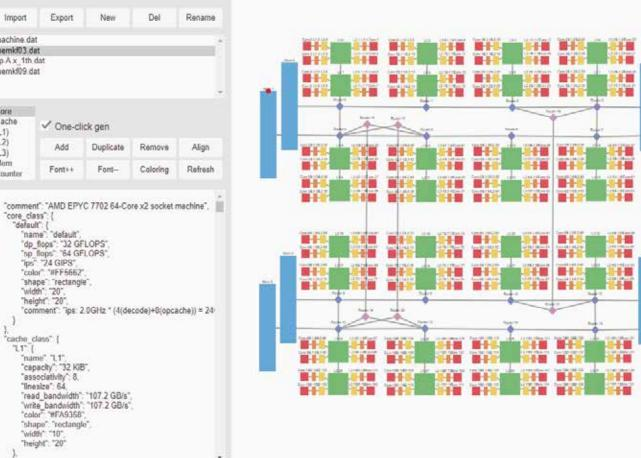
GUI tool to describe the architecture to be estimated. The user describes the memory hierarchy as a graph that consists of memory objects, caches and CPU cores.
