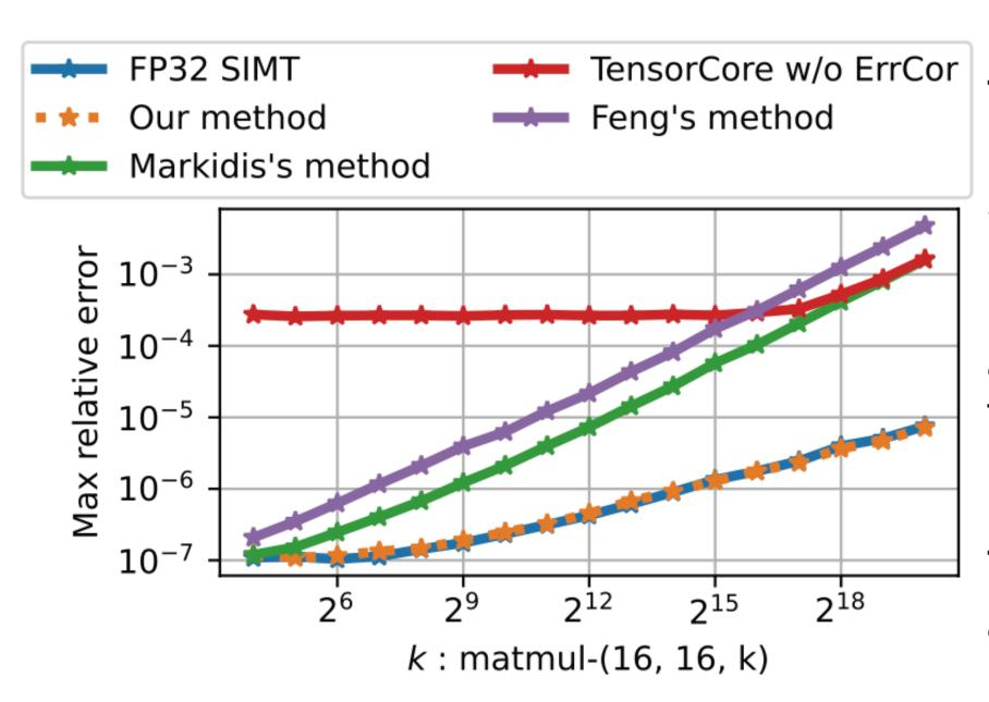
TensorCores multiply two 16bit matrices and accumulate into a 32 bit matrix. This conversion to 16bit results in a significant loss in precision. The use of an auxiliary 16bit matrix to store the mantissa loss is known to partially correct this error. However, the round-to-zero in TensorCore accumulation is another source of error that has not been accounted for in
