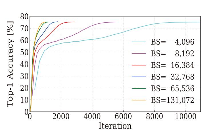
Data-parallel training of deep neural networks suffers from the large-batch problem, where the generalization gap increases as the mini-batch size increases proportional to the number of GPUs. Using the Kronecker Factorization mention on the right, we are able to use a second order optimization method with minimum
