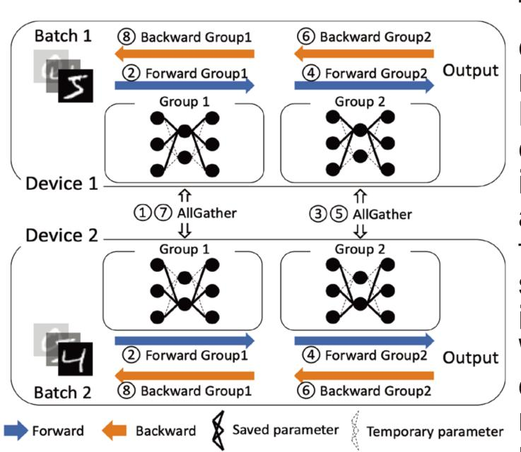
The size of deep neural networks continues to grow rapidly, where models like GPT-3 and Megatron-LM exceed the memory capacity of a single GPU. The trend in computer architecture where the arithmetic throughput is growing faster than memory capacity, suggests that memory consumption is a critical issue in deep learning. We reduce the memory usage of deep neural networks by scattering, recomputing, and offloading the model parameters and activations.
