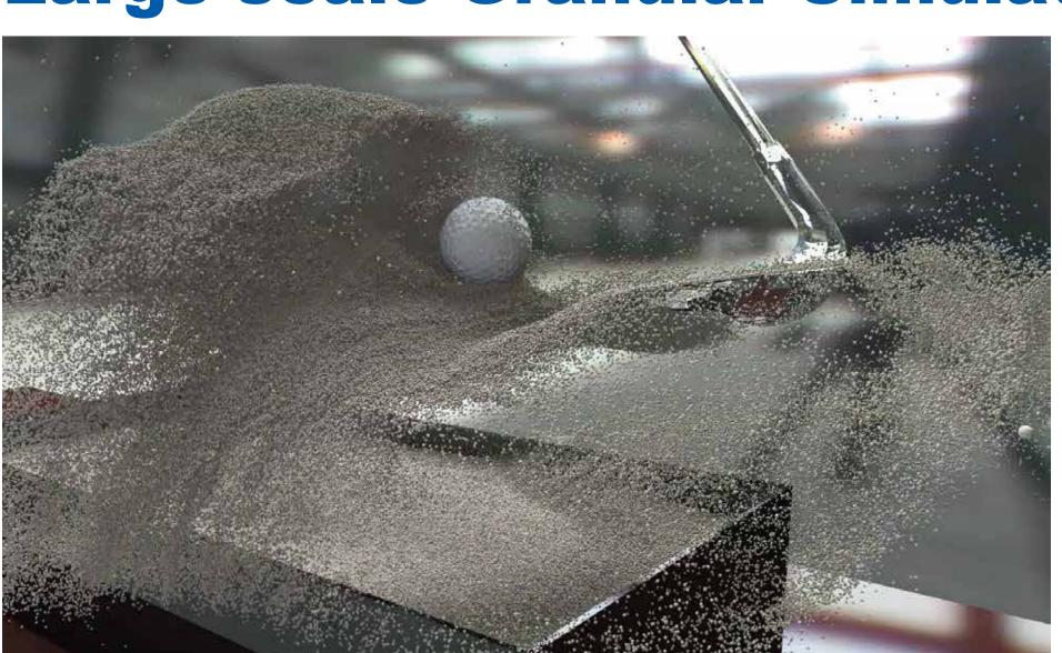
Discrete element method (DEM) is often used to simulate granular dynamics and its simple algorithm with the contact interaction is suitable for GPU computing. However so many particles are included and the particle distributions are changing in time and space. A dynamic domain
