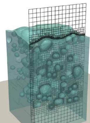
Foam formation with a stable thin liquid film is very difficult to simulate using conventional methods due to the limitation of mesh resolution that can be used. We
