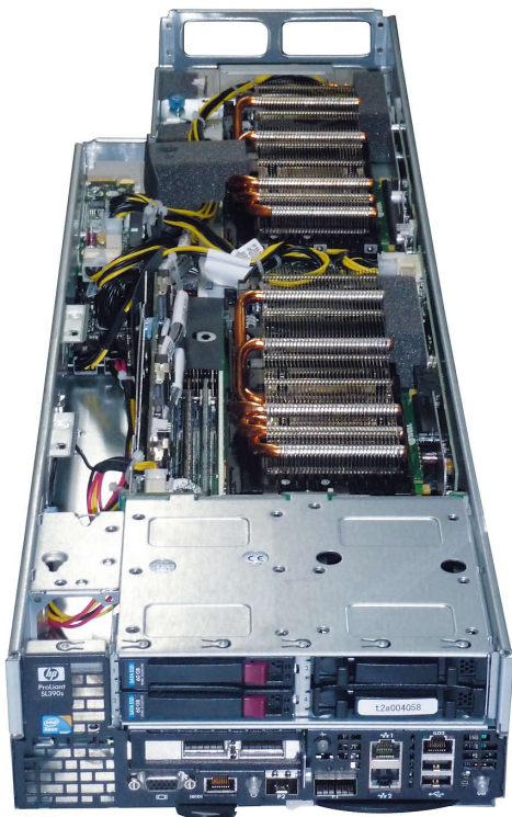
Figure 6 Individual compute nodes in TSUBAME2.0 are 1/4th the size of TSUBAME1 nodes, despite being 10 times more computationally powerful.
