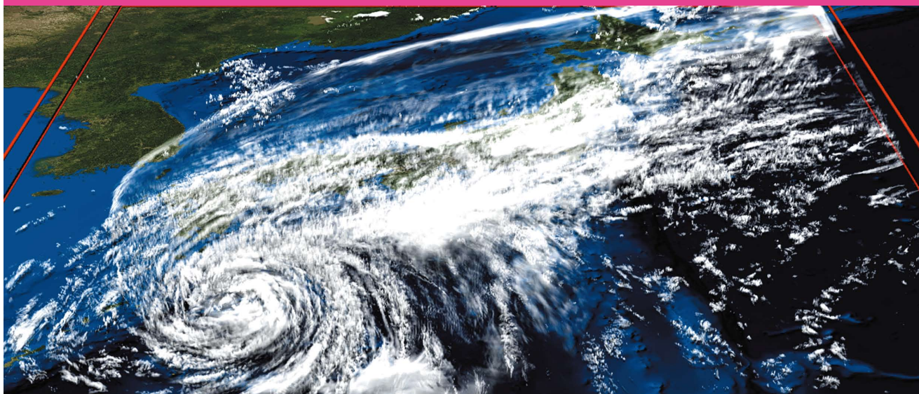
Figure 6 ASUCA real operation to describe a typhoon with 4792 \times 4696 \times 48 mesh using 437 GPUs of TSUBAME 2.0
