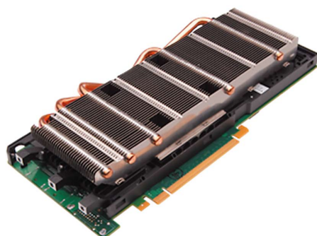
Figure 4 NVIDIA Tesla M2050 GPU used in TSUBAME2.0, 3 cards per node, over 4000 cards in total.
