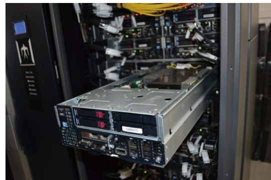
Fig. 2 Compute node of TSUBAME2.5 embodying the new NVIDIA Kepler K20X GPU
