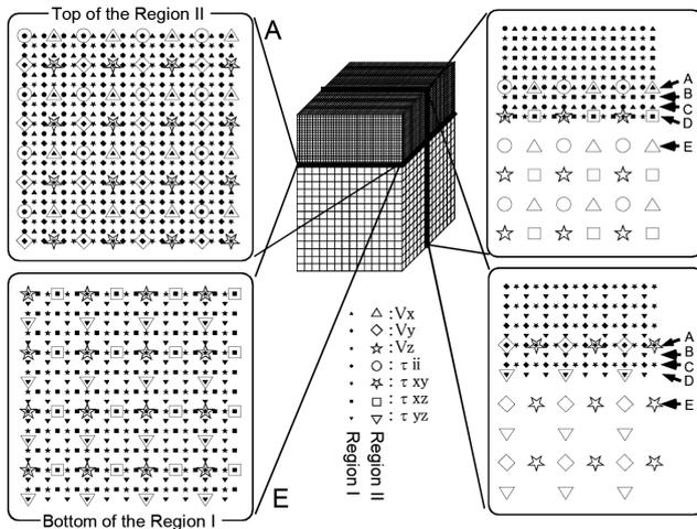
**Fig. 1** (center) 3-D discontinuous grid system. (left) Two transactions on the top and at the bottom of the overlapping region of Regions I and II, where the elimination or the insertion of grid points is necessary. (right) Two profiles of the discontinuous grid.
