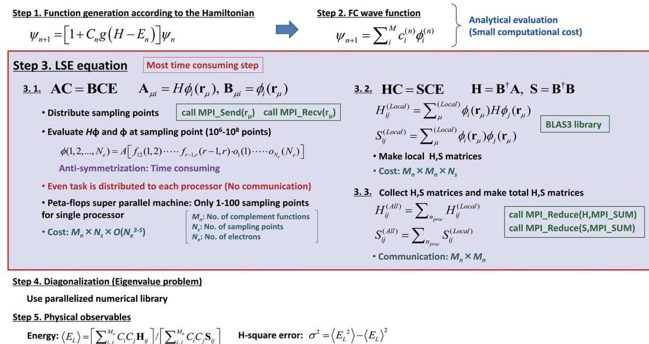
Fig. 2 Parallel algorithm of the FC-LSE method
