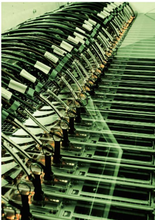
**Fig. 4** The compute nodes submerged in the GRC Carnot Jet system.
