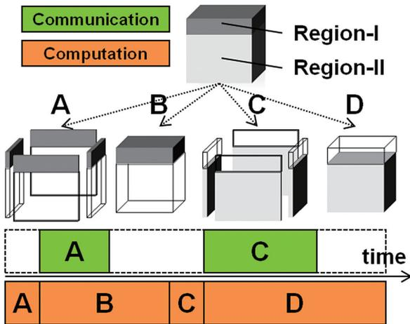
Fig. 3 Popular method for concealing the communication. The values on the overlapped grids are antecedently calculated to other grids.
