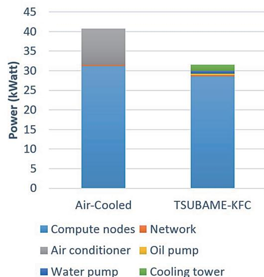
Fig. 6 PUE Evaluation of TSUBAME-KFC versus air-cooled system
